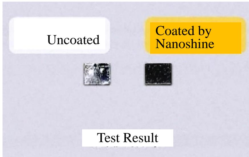
High Pressure Washing Test with Aluminum Plate
