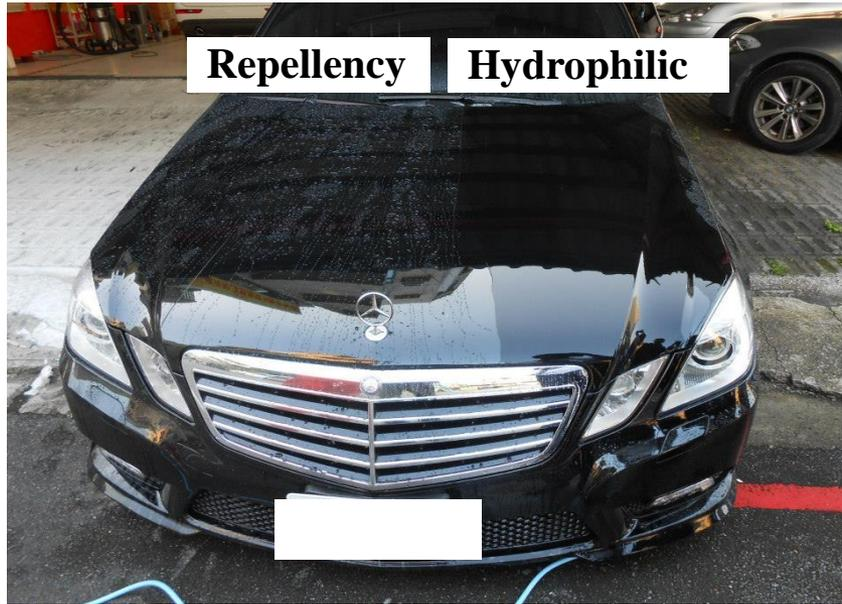
Comparison Between Hydrophilic and Repellency on a Car Body
