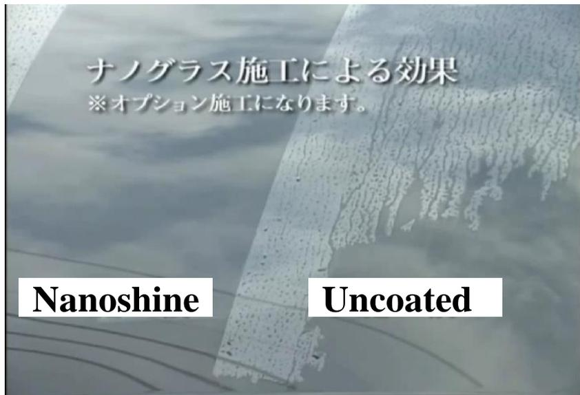
Comparison Between Coated Nanoshine and Uncoated with Windowpane on a car body
