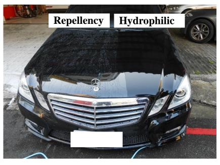
Comparison Between Hydrophilic and Repellency on a Car Body
